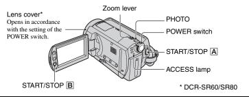
**1** Slide the POWER switch in the direction of the arrow repeatedly to light up the respective lamp.
