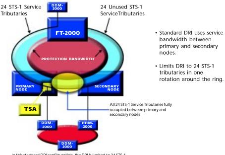
In this standard DRI configuration, the DRI is limited to 24 STS-1 tributaries in one rotation around the ring.
