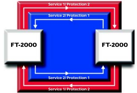
The FT-2000 OC-48 Add/Drop-Ring Terminal supports two-fiber bi-directional line-switched rings. The rings are standards-compliant and support the maximum number of nodes allowed by the SONET standard — 16 nodes. They perform automatic protection switching, restoring traffic in 60 milliseconds or less for catastrophic failures in rings without existing switches and extra traffic.
