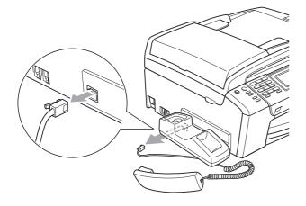
2 Pull the tab (1) back and hold it in position as you push the cradle (2) to the back of the machine.
