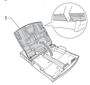
3 With both hands, gently press and slide the paper side guides (1) and paper length guide (2) to fit the paper size. Make sure that the triangular marks (3) on the paper side guides (1) and paper length guide (2) line up with the mark for the paper size you are using.
