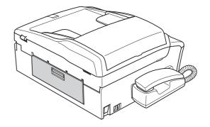
6 Lift the scanner cover (1) from the front side of the machine until it locks securely into the open position. Make sure that there is no jammed paper left inside the machine.
