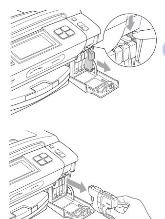
Open the new ink cartridge bag for the color shown on the LCD, and then take out the ink cartridge.
