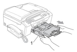
Pull out the jammed paper (1) and press Stop/Exit.
