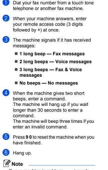
If your machine is set to Manual mode and you want to use the remote retrieval features, wait about 100 seconds after it starts ringing, and then enter the remote access code within 30 seconds.
