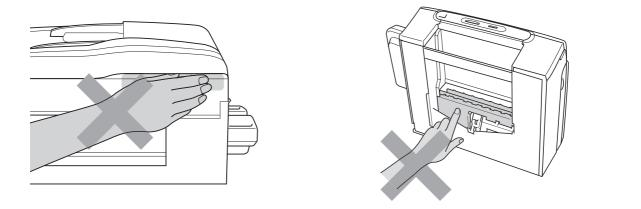
When moving the machine you must lift it from the base, by placing a hand at each side of the unit as shown in the illustration. DO NOT carry the machine by holding the scanner cover or Jam Clear Cover.
