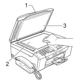
2 In the ADF unit, clean the white bar (1) and the glass strip (2) with a lint-free cloth moistened with a non-flammable glass cleaner.
