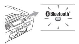
You can print photos only when the indicator is illuminated in blue. (For details about turning on the indicator, see *Enable Bluetooth<sup>®</sup> wireless technology on your machine* on page 125.)
