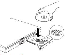
Inserting a disc
