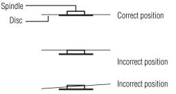
Positioning the disc on the spindle
