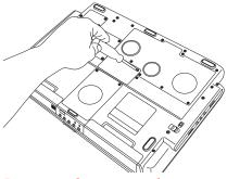
Removing the memory slot cover
