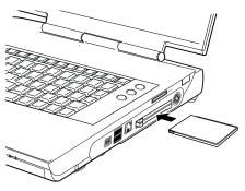
Inserting a PC Card
