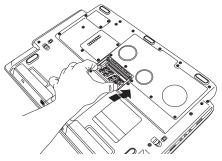
Inserting the memory module
