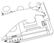
Sample pushing and holding the battery release latch
