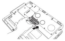
Sample inserting the memory module
