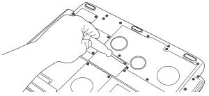
Sample removing the memory module slot cover screws
