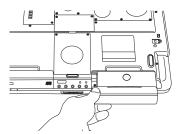
Sample sliding the battery out
